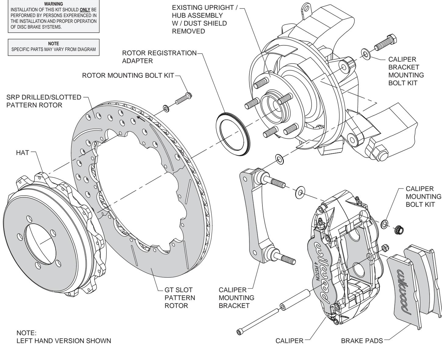
**Typical Installation Diagram (2008-2012 Subaru WRX Kit Shown)**
